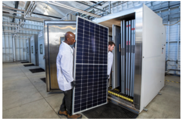
Extended reliability testing at PVEL's Berkeley Lab
